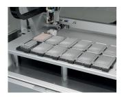
High speed XYZ axes, top speed: 1000 mm/s
