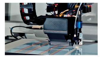
**Bulk Mode** uses onboard reservoirs to supply each channel directly, enabling continuous operation with minimal fluid handling. It offers maximum stability, cleanliness, and speed for high-volume production, while eliminating any risk of cross contamination.
