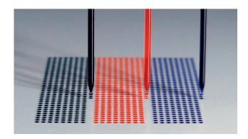
Aspirate / Dispense Mode is ideal when precise control of multiple reagents across different and diverse samples is needed. Each channel draws liquid from any reservoir, such as wells, tubes, or custom containers, before dispensing it in full synchronization.
